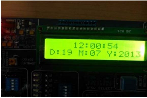
Fig. 25 Photograph of PCF8583 Interfacing
